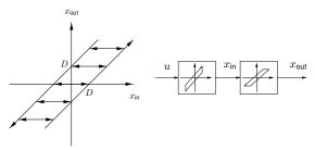
ldea: Let  $x_{\rm in}$  jump  $\pm 2D$  when  $\dot{x}_{\rm out}$  should change sign. Works if the backlash is directly on the system input!
