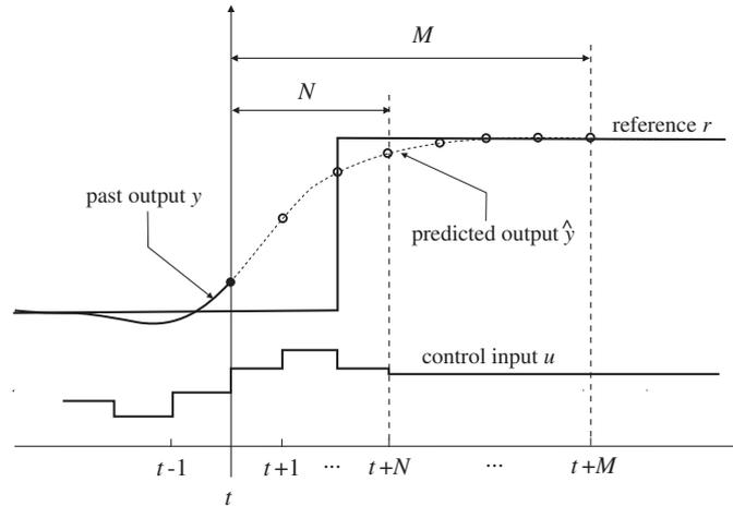
**Figure 2** Illustration of the receding horizon principle used in Model Predictive Control.
