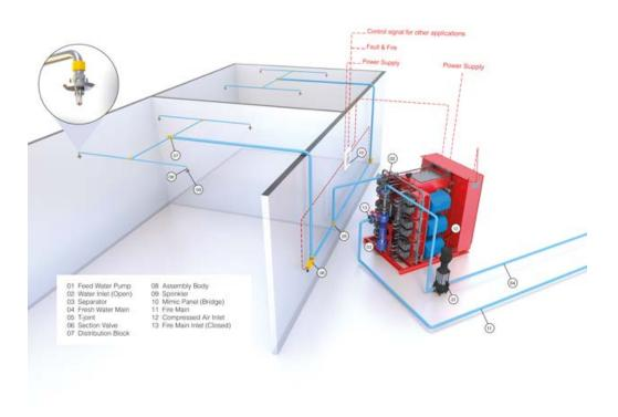
Wet pipe system uses automatic sprinklers attached to a piping system containing water and connected to a water supply so that the water discharges immediately from sprinklers operated by the heat from a fire. Wet pipe systems are typically used in accommodation and similar areas with solid combustibles.
