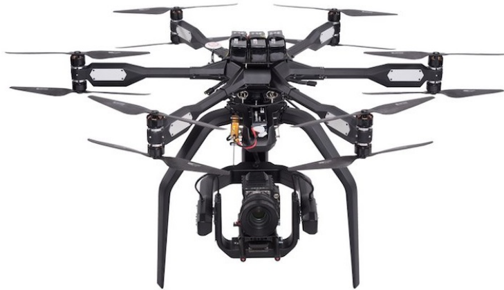
Figure 1.1: Intuitive Aerial AB in Linköping develops a camera-carrying Hexacopter. For high-precision autonomous flight (and filming), it is important to know the orientation (pitch-, roll- and yaw-angles) of the system. Gyros and accelerometers are used to extract as much information as possible, with as little error and noise as possible.
