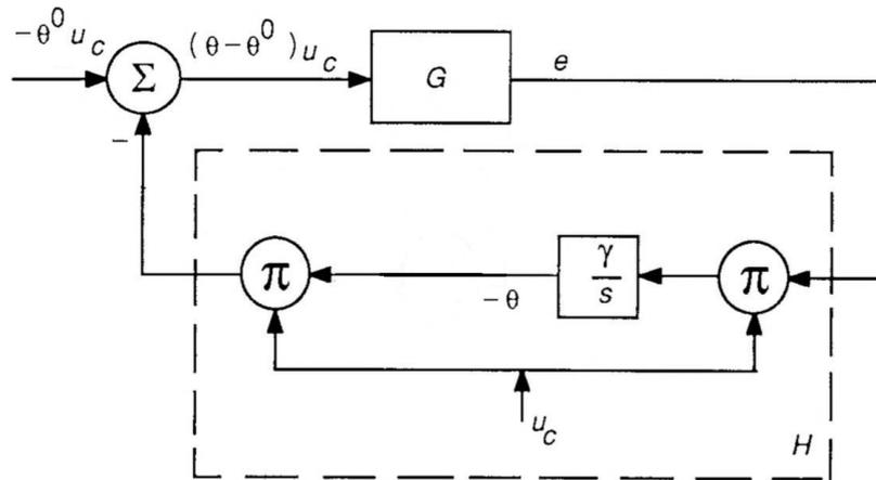
**Figure 3** A model-reference adaptive system where the feedforward gain  $\theta$  is adapted.
