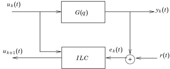
Figure 2 An ILC feedback system.
